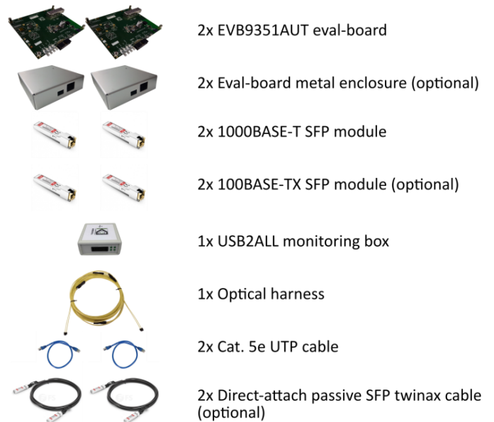
Figure 4. Typical content of an EVK9351AUT eval-kit
